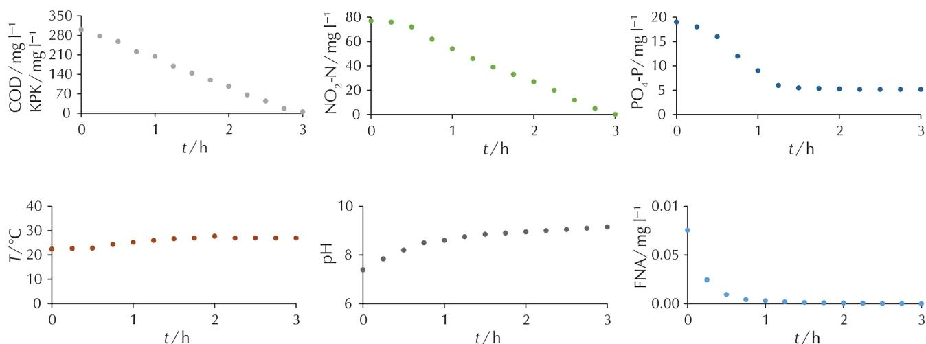
Fig. 1 – Variations of COD,  $\text{NO}_2\text{-N}$ ,  $\text{PO}_4\text{-P}$ , FNA, temperature, and pH in batch test with 80 mg  $\text{NO}_2\text{-N/l}$  at N/P ratio of 4 and C/N ratio of 2
