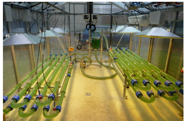
Fig. 3 – Cultivation systems for photo-autotrophic microorganisms: open cascade system (top – © Jiri Kopecky, Institute of Microbiology), closed tubular photobioreactor at pilot-scale (bottom – © Katharina Meixner, IFA Tulln/University of Natural Resources and Life Sciences)
