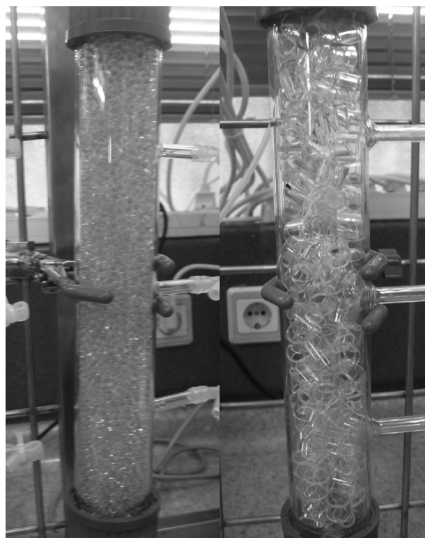
Fig. 1 – Glass Beads and Glass Rushing Rings support materials and plug flow fermentor view before immobilization process for continuous 1,3-PDO production
