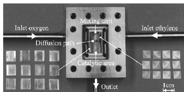
Fig. 3 – Microreactor ethylene oxide synthesis. Reprinted with permission.<sup>39</sup> Copyright (2002) American Chemical Society.
