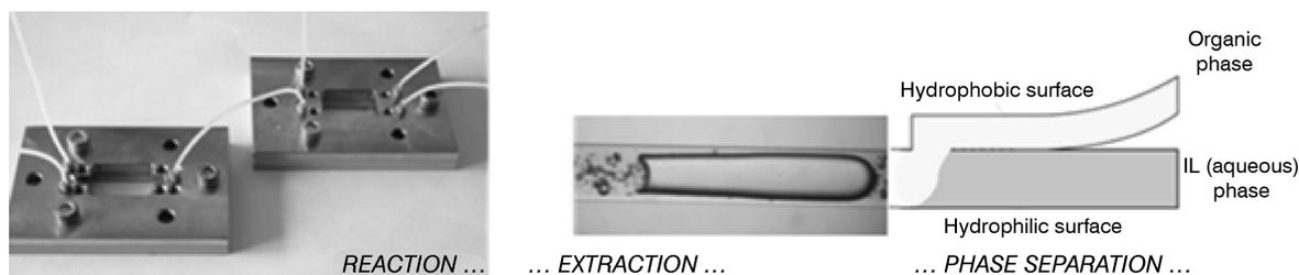
Fig. 6 – Scheme of an integrated microchemical system representing a consecutive reaction, extraction and phase separation
