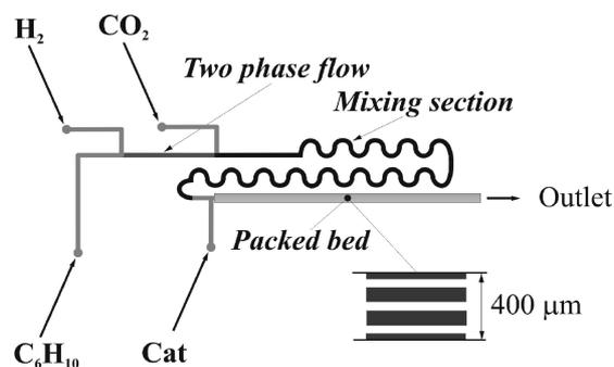
Fig. 1 – Packed bed microreactor<sup>36</sup> – schematic of the channel design
