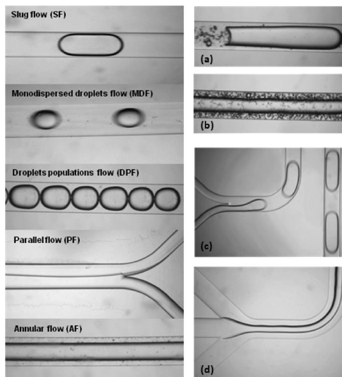
Fig. 4 – Flow patterns for two immiscible fluids
