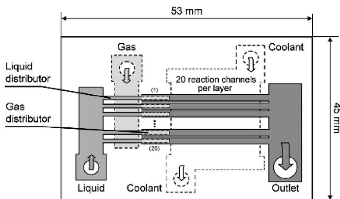
Fig. 5 – Microreactor for fast gas-liquid reactions. Reprinted with permission.<sup>57</sup>
