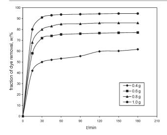
Fig. 5 – Effect of adsorbent mass on the adsorption of dye on SDC (Dye mass concentration  $\gamma_d = 250$  mg  $L^{-1}$ , volume of sample V = 100 ml, pH 7.0)
