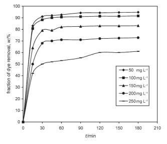
Fig. 3 – Effect of initial dye mass concentration on the adsorption of rhodamine-B on SDC (adsorbent dose  $\gamma_{ad} = 4.0 \text{ g } l^{-l}, \text{ pH 7.0}$ )
