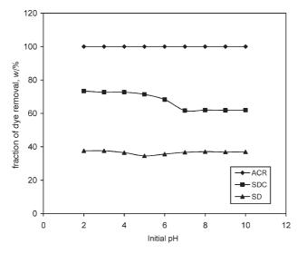
Fig. 2 – Effect of pH on dye mass adsorption (Dye mass concentration  $\gamma_d = 250 \text{ mg } L^{-l}$ , adsorbent dose  $\gamma_{ad} = 4.0 \text{ g } l^{-l}$ , equilibrium time t = 3 h)
