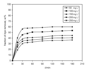
Fig. 4 – Effect of initial mass concentration on the adsorption of rhodamine-B on SD (adsorbent dose  $\gamma_{ad}$  = 4.0 g  $l^{-l}$ , pH 7.0)
