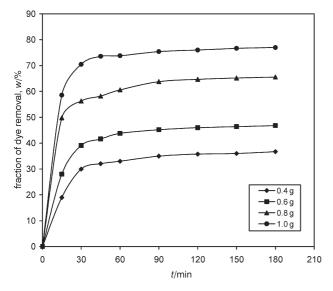
Fig. 6 – Effect of adsorbent mass on the adsorption of dye on SD (Dye mass concentration  $\gamma_d = 250 \text{ mg } L^{-1}$ , volume of sample V = 100 ml, pH 7.0)
