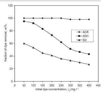
Fig. 1 – Effect of adsorbent change on dye removal (pH 7.0, adsorbent dose  $\gamma_{ad} = 4.0$  g  $l^{-l}$ , equilibrium time, t = 3 h)
