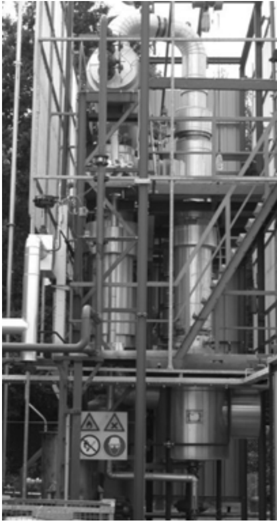
Fig. 4 – Photograph of the TU Delft total reflux distillation column
