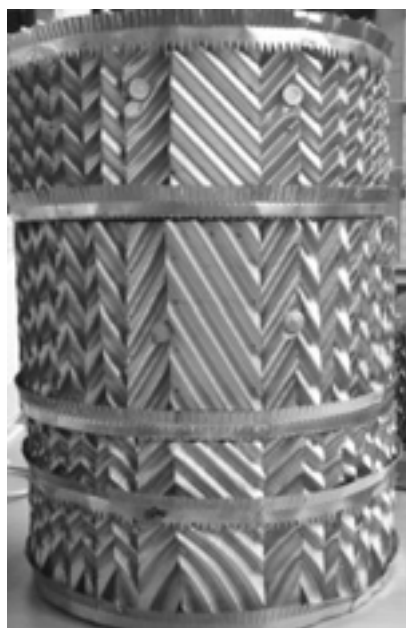
Fig. 1 – Photograph of 0.45 m diameter elements of common size B1-series packings with inclination angles of 45 and 60 degrees, respectively, and the bend in the bottom part (B1-250M) of corrugated sheets
