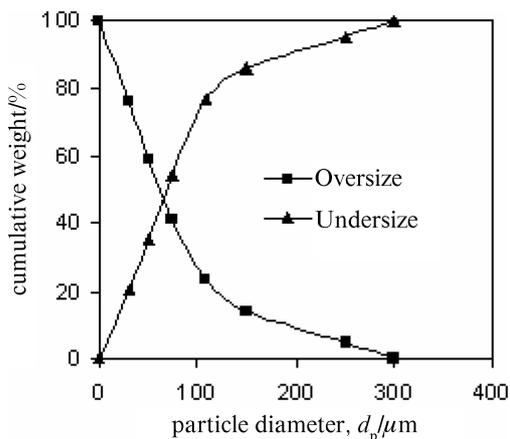
Fig. 2 – Particle diameter distribution of calcite samples
