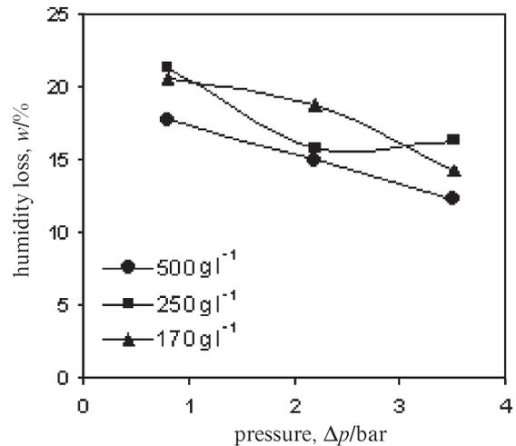
Fig. 7 – Variation of humidity loss against different initial suspension concentrations and filtration pressures
