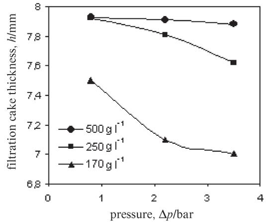
Fig. 6 – Variaton of filter cake thickness against different initial suspension concentrations and filtration pressures
