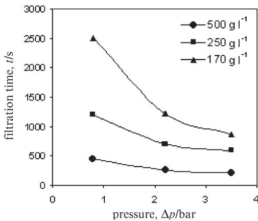
Fig. 5 – Variation of filtration time against different initial suspension concentrations and filtration pressures
