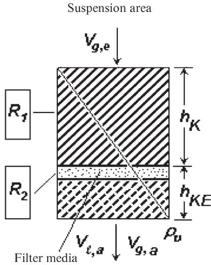
$V_{g,e}$  = suspension volume       $\rho_o$  = suspension density
