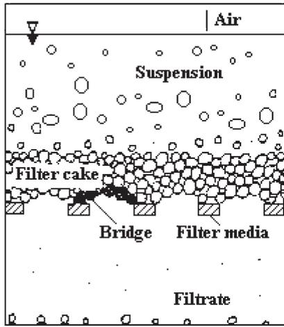
Fig. 1 – Occuring of the particle bridge on the filter cloth
