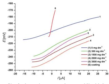
Fig. 2 – Linear polarization curves for copper in 0.51 mol dm<sup>3</sup> NaCl solution without stirring as a function of various propolis extract concentrations
