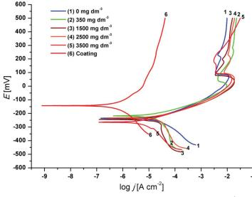
Fig. 3 – Potentiodynamic polarization curves in 0.51 mol dm<sup>-3</sup> NaCl solution as a function of various propolis extract concentrations
