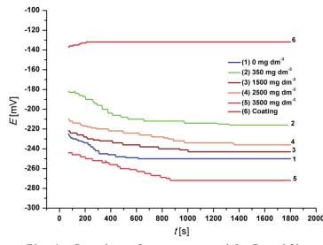
Fig. 1 – Dependence of corrosion potential for Cu in 0.51 mol dm<sup>3</sup> NaCl solution in the absence and presence of propolis extract as a function of time
