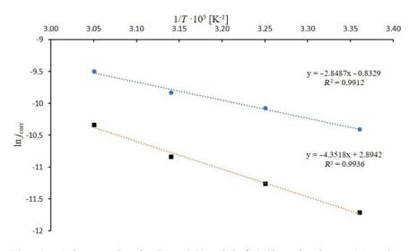
Fig. 5 – Arrhenius's plots for Cu in 0.51 mol  $dm^{-3}$  NaCl: in the absence (•), and in presence of propolis extract (**1**) in concentration of 3500 mg  $dm^{-3}$
