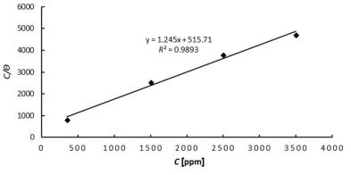
Fig. 4 – Langmuir's adsorption isotherm for propolis adsorption process on the copper surface in NaCl solution
