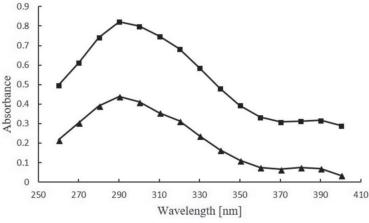
Fig. 6 – UV-Visible spectra of test solution with propolis extract (3500 mg dm<sup>-3</sup>): before immersion ( $\bullet$ ), and after 48 hours immersion ( $\bullet$ ) of copper samples in solution
