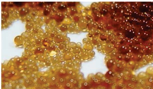
Fig. 1 – Wet particles of the ion exchanger before drying
